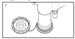
4. When air flows out the back of the inflator, the desired pressure has been achieved. Remove inflator and tightly secure valve cap.
