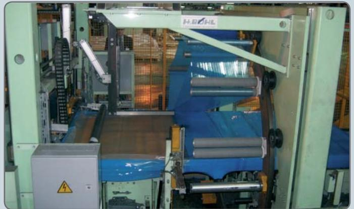
Our machine design with automatic product height registration to secure a constant lay on force in combination with the memory effect of stretch film maintains the high tension and stability of the unit, even where a pack shrinks as the product cools.
