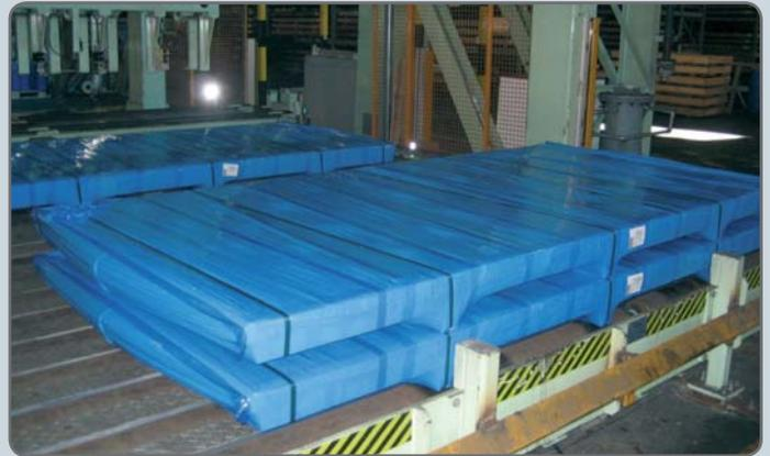
For cold and hot rolled material with or without pallets - The FLATPACK machine protects your goods. Inline solution in combination with the cut to length line.
